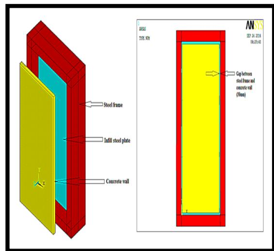
Figure 2: Composite steel plate shear wall(numerical )
