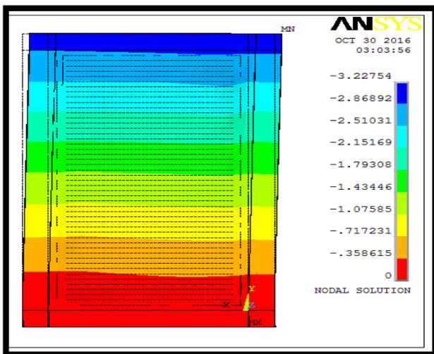
Figure 9: Out-of plane deflection of CSPW for 55 MPa
