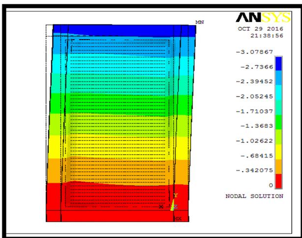
Figure 10: Out-of plane deflection of CSPW for 65 MPa
