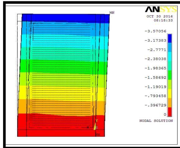
Figure 5: Out-of plane deflection of CSPW for 25 MPa
