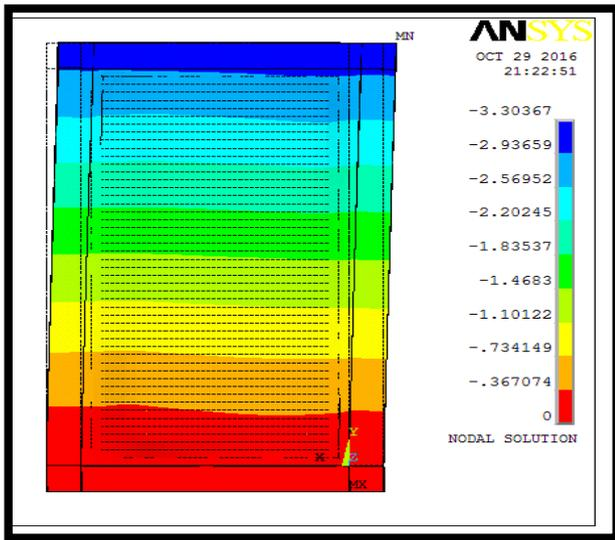
Figure 8: Out-of plane deflection of CSPW for 50 MPa
