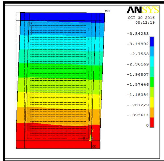
Figure 6: Out-of plane deflection of CSPW for 28 MPa
