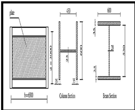
Figure 1: Specimen dimensions
