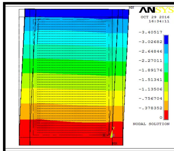
Figure 7: Out-of plane deflection of CSPW for 45 MPa
