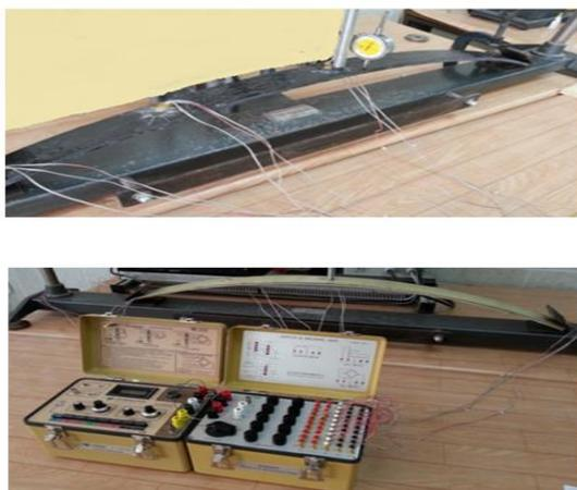
Figure 6: Application of rectangular rosette strain gauges in different modes of composite Shells under bending test
