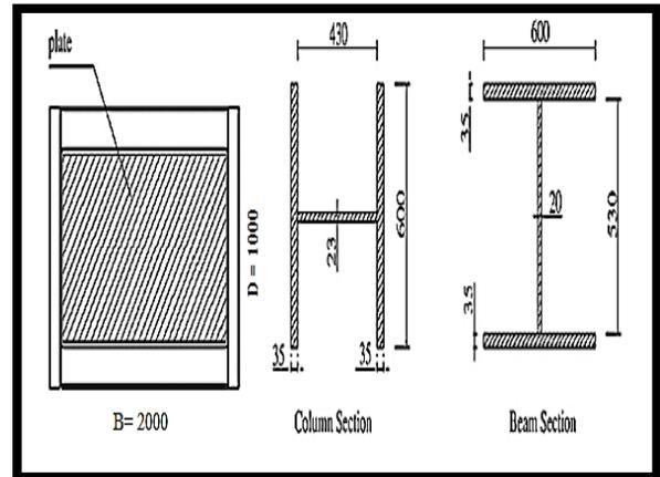
Figure 2: Specimen dimensions
