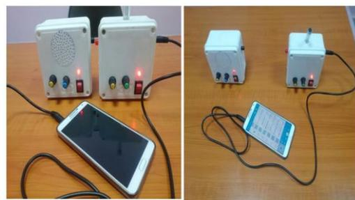
Figure 8: The circuit working of IR-communication system
