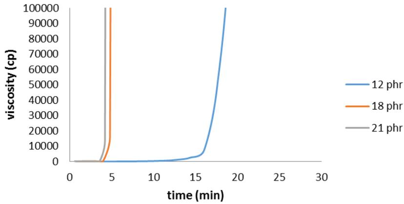
Figure 6. Viscosity vs gel time with differ cure composite at 100 °C.
