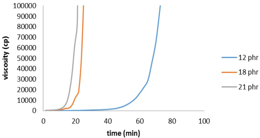
Figure 4. Viscosity vs gel time with differ cure composite at 80 °C.
